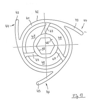
[9] In the embodiment of Figure 12, the shell part 42 is elastically deformable, and is also connected to the hexagonal hub through resilient spokes 47 (in fact the spokes are more like walls as they have axial length, but the specification calls them spokes). This creates what are described as deformation chambers 49, which can be compressed during operation of the rollers. ..
